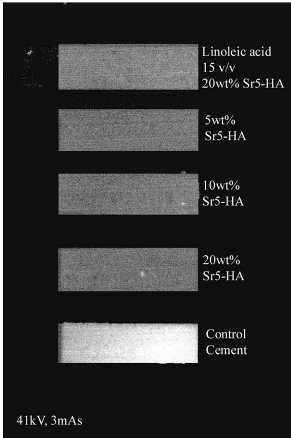
**FIGURE 1.** Radiopacity of (a) 5 wt % Sr5-HA, (b) 10 wt % Sr5-HA, (c) 20 wt % Sr5-HA, (d) 20 wt % Sr5-HA with 15 v/v linoleic acid, and (e) control bone cement taken at 41 kV and 1.8 mAs.
