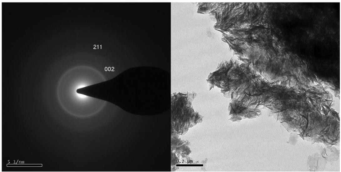
**FIGURE 4.** TEM and SAED pattern of precipitated particle deposited on 20 wt % Sr5-HA cement surface after 14 days; the coating was easily scratched from the surface after cleaning and drying.
