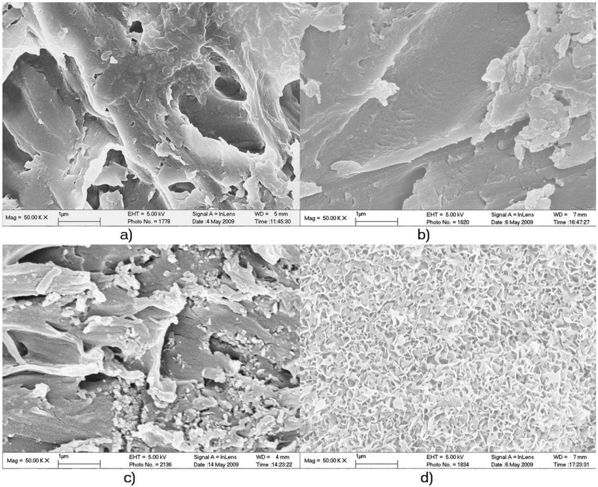
**FIGURE 3.** Surface morphology of bone cements before and after immersed in SBF at 37°C for 14 days: (a) control cement and (b) 5 wt % Sr5-HA, (c) 10 wt % Sr5-HA, (d) 20 wt % Sr5-HA, and (e) 20 wt % Sr5-HA with 15 v/v linoleic acid.
