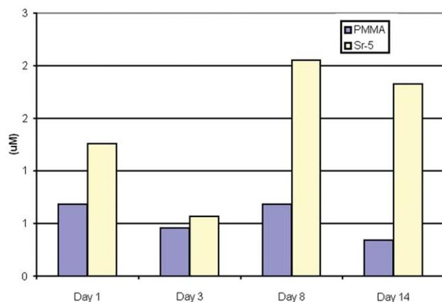
**FIGURE 5.** Strontium concentration of control cement and 20 wt % Sr5-HA bone cements after soaking in SBF at 37°C for 1, 3, 8, and 14 days. [Color figure can be viewed in the online issue, which is available at [wileyonlinelibrary.com](http://wileyonlinelibrary.com).]
