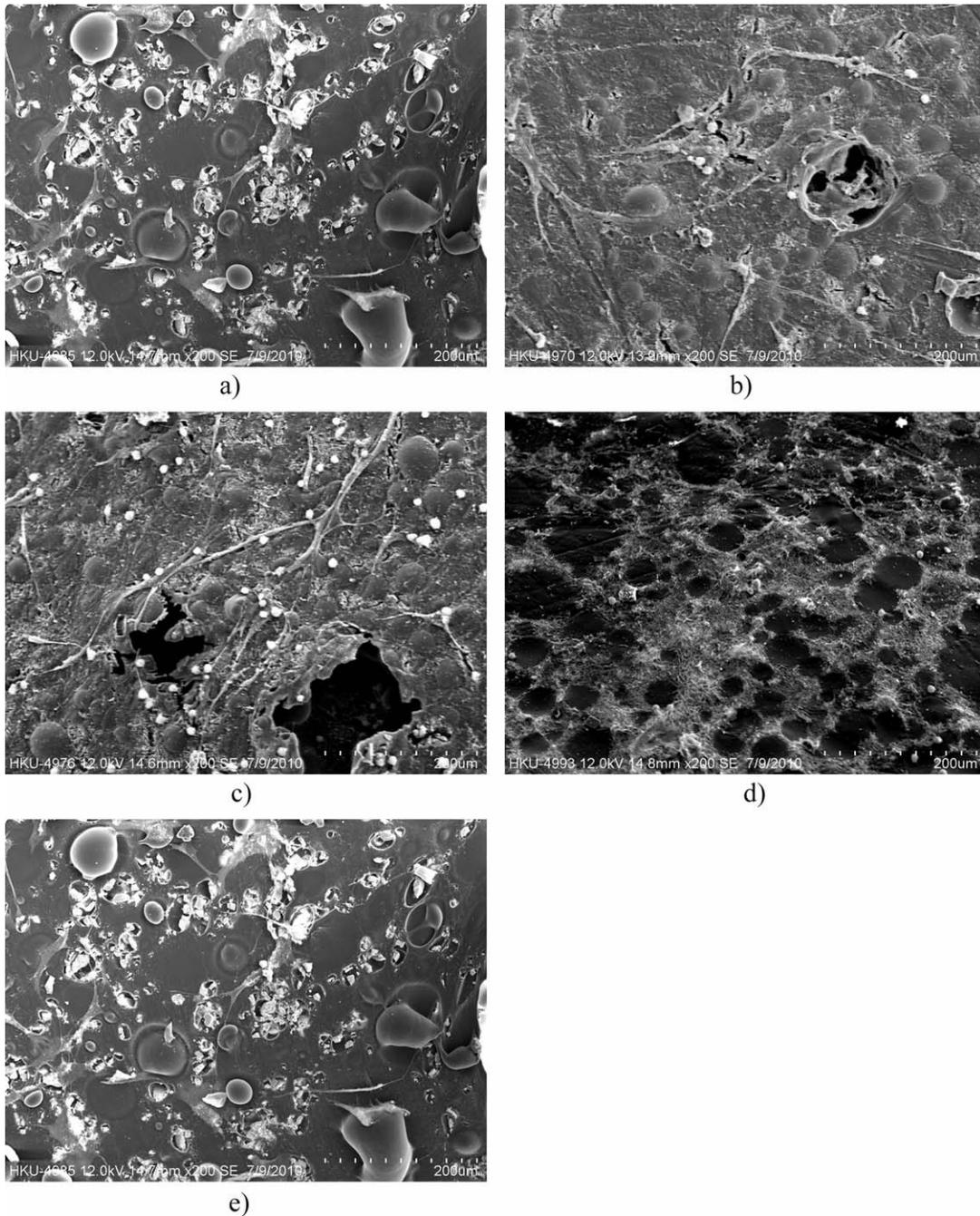
**FIGURE 6.** SEM image of cell adhesion on control bone cements and (a) 5 wt %, (b) 10 wt %, (c) 20 wt % Sr5-HA, (d) 20 wt % Sr5-HA with 15 v/v linoleic acid bone cement, and (e) control cement surface seeded with MC3T3-E1 respectively for 3 days.
