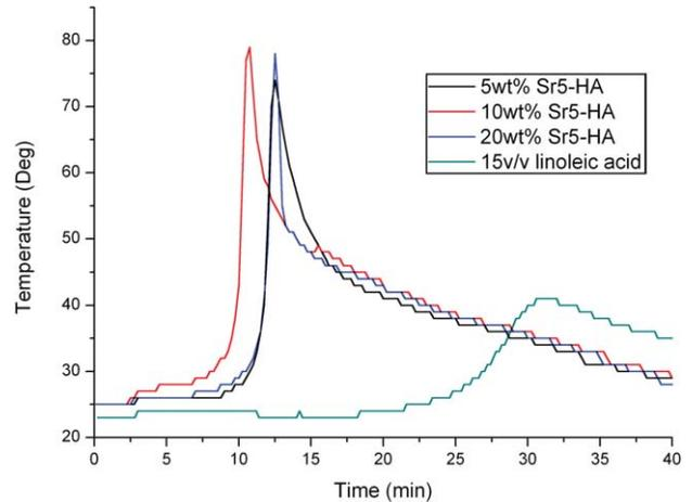
**FIGURE 2.** Setting curve of (a) 5 wt % Sr5-HA, (b) 10 wt % Sr5-HA, (c) 20 wt % Sr5-HA, and (d) 20 wt % Sr5-HA with 15 v/v linoleic acid bone cement. [Color figure can be viewed in the online issue, which is available at [wileyonlinelibrary.com](http://wileyonlinelibrary.com)]
