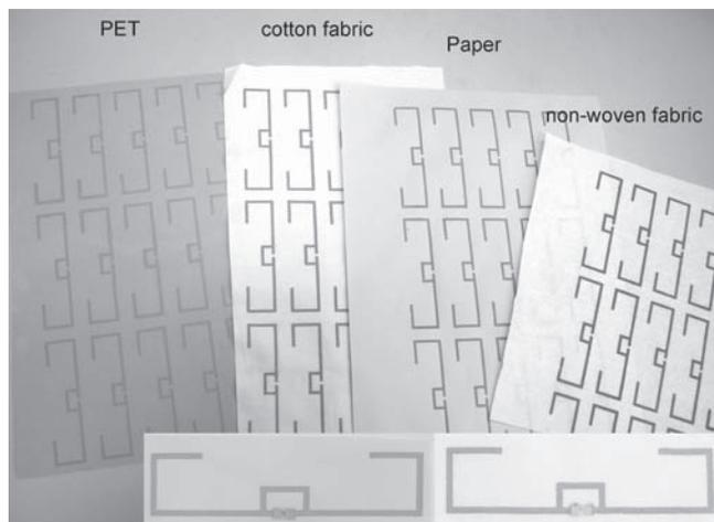
**Figure 6.** A photograph showing some of the RFID antennas which were printed on various substrate materials, including PET, cotton fabric, paper, and non-woven fabric. The two insets are the RFID tag samples on paper (left) and cotton fabric (right). The straps were attached to the antenna immediately after the antenna printing process.
