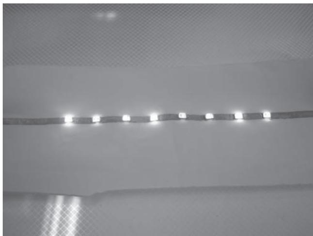
**Figure 5.** A photographic image of a piece of WBICA printed circuit line (2 mm x 150 mm) which supports 8 LED chips in different color. (Ag: 80 wt%, NaBH<sub>4</sub>: 0.5%).
