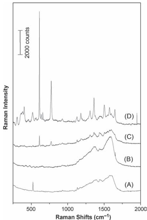
**Figure 3.** Raman scattering of the silver flake samples with the chemisorbed R6G. A) original silver flake sample; B) iodine treated silver sample; C) 0.5%  $\text{NaBH}_4$  treated iodinated silver flake sample, and D) 1%  $\text{NaBH}_4$  treated iodinated silver flake sample.
