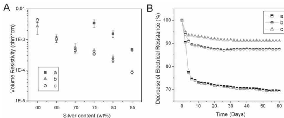
**Figure 4.** A) Volume resistivity of the WBICAs versus different addition amount of NaBH<sub>4</sub>: a) no NaBH<sub>4</sub> addition; b) 0.5% of NaBH<sub>4</sub>; c) 1% of NaBH<sub>4</sub>. B) Temperature-humidity reliability of the WBICAs versus aging time: a) no NaBH<sub>4</sub> addition; b) 0.5% of NaBH<sub>4</sub>; c) 1% of NaBH<sub>4</sub>.
