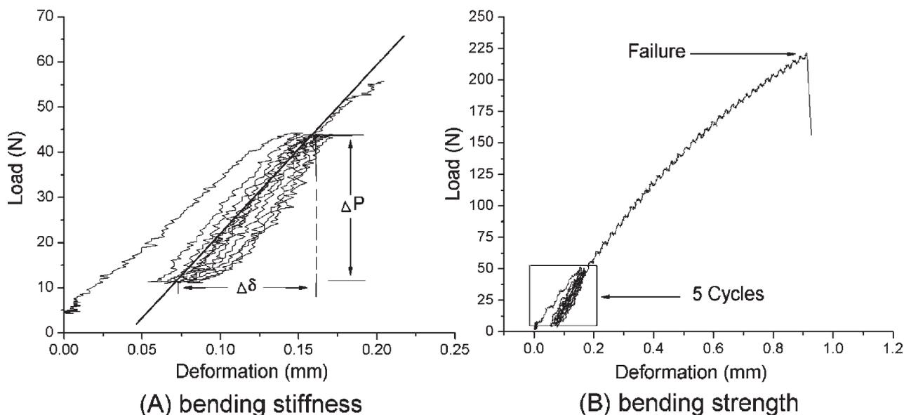
**Figure 1.** Bending test curves of original Sr-HA bone cement. A: Five cycles of loading were applied, and linear regression was used to calculate stiffness;  $\Delta P$  is the force applied,  $\Delta\delta$  is the deformation; B: Bending curve for strength determination.
