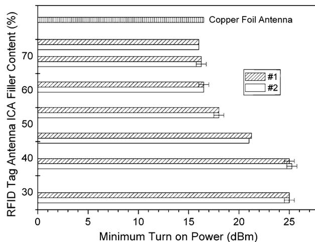
Fig. 8. Minimum turn-on power of the reader to detect the RFID tags with the antenna printed using the ICAs, compared with the read range performance of control metal foil-based RFID tag samples.
