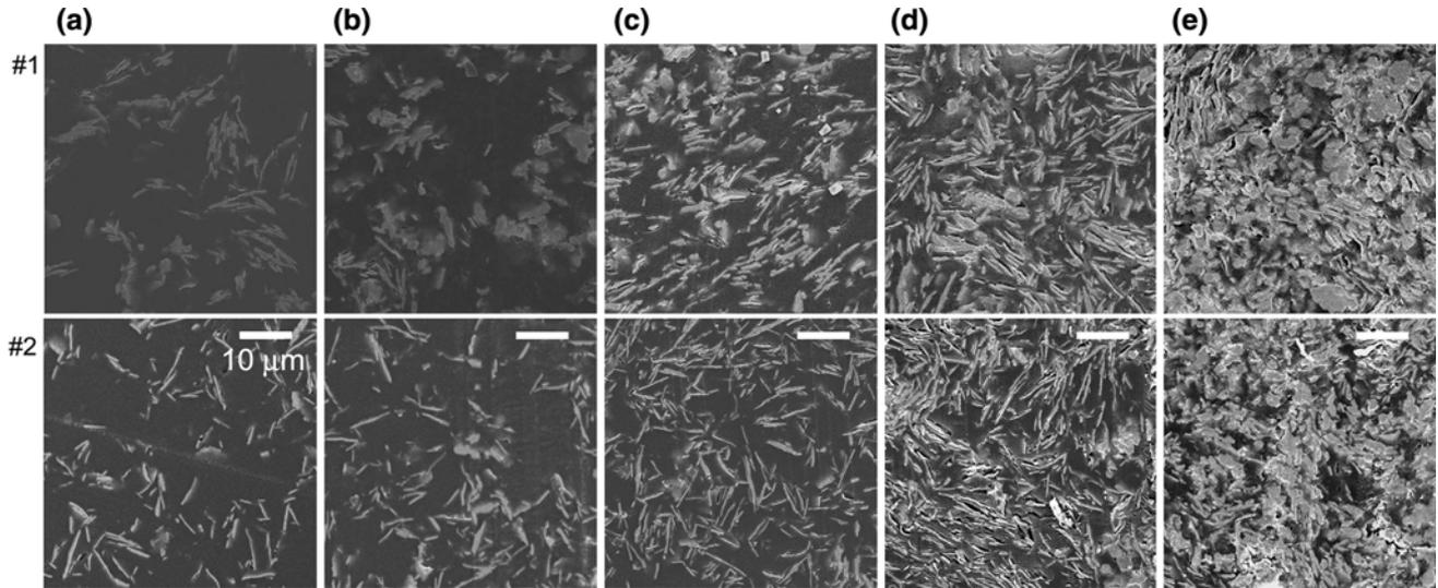
Fig. 2. SEM images of cross-sections of some of the ICA bulk samples: (a) 30% filler, (b) 40% filler, (c) 55% filler, (d) 70% filler, and (e) 75% filler (scale bars = 10 μm).
