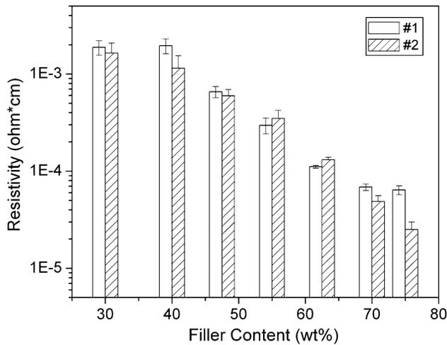
Fig. 3. Resistivity of printed resistors of ICAs (series 1 and 2) with different silver filler contents.
