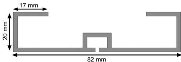
Fig. 7. Designed geometry of RFID tag antenna based on the ICA paste with 30 wt.% silver content.
