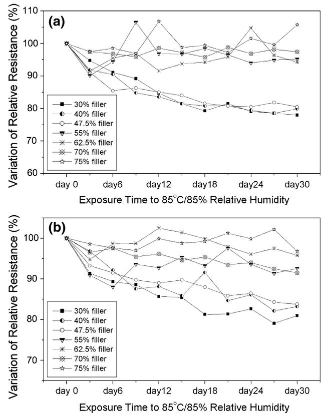
Fig. 4. 85°C/85% relative humidity reliability analysis of the ICAs (resistance measurement). (a) Variation of the relative resistance of the printed resistors of ICA series 1. (b) Variation of the relative resistance of the printed resistors of ICA series 2.
