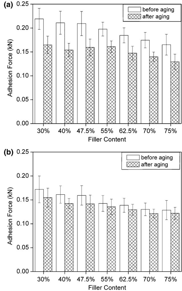
Fig. 6. 85°C/85% RH reliability analytical result of the ICAs (lap shear mechanical force measurement). (a) Variation of the lap shear adhesion force of ICA series 1 onto PET substrates. (b) Variation of the lap shear adhesion force of ICA series 2 onto PET substrates.
