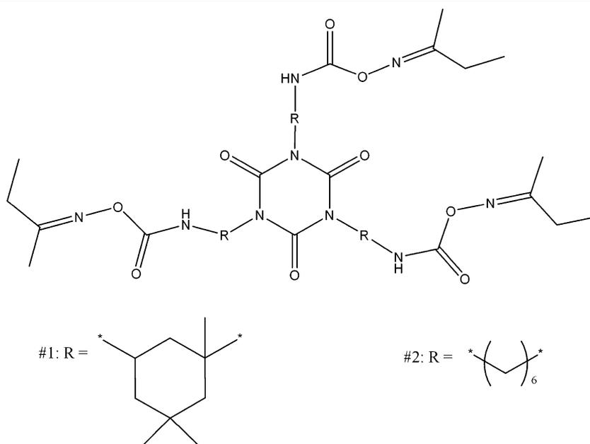
Fig. 1. Structure of the blocked polyurethane prepolymers for series 1 and 2.
