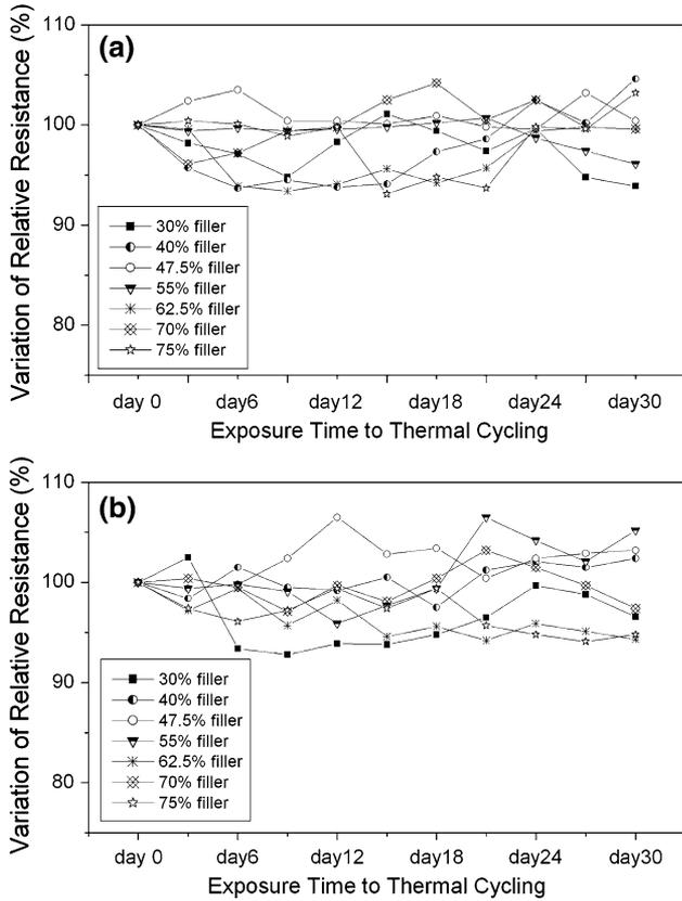
Fig. 5. Thermal cycling analysis of the ICAs. (a) Variation of the relative resistance of the printed resistors of ICA series 1. (b) Variation of the relative resistance of the printed resistors of ICA series 2.
