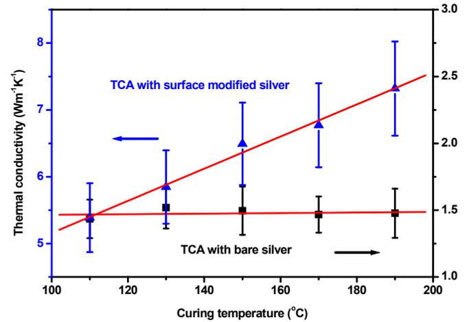
**Fig. 5 Thermal conductivity of TCA with at 80 wt% filler concentration in various curing temperatures (the curing duration for 110 °C is 2 hours and the others are 30 minutes; Blue: TCA with modified silver fillers, Black: TCA with bare silver fillers)**
