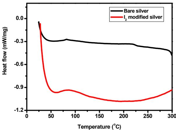
**Fig. 4 DSC curves of the silver particles**
