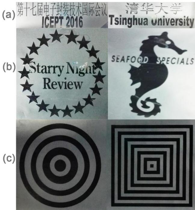
Fig.4 photographic images of various designable electrode designs. (a) Words and letters. (b) Different kinds of patterns. (c) Planar electrode arrays.
