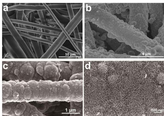
Fig. 2. (a) SEM images of polymer fiber. (b) SEM image of nickel coated polymer fiber. (c), (d) SEM image of MnO<sub>2</sub> deposited on nickel coated polymer fiber with different magnification.
