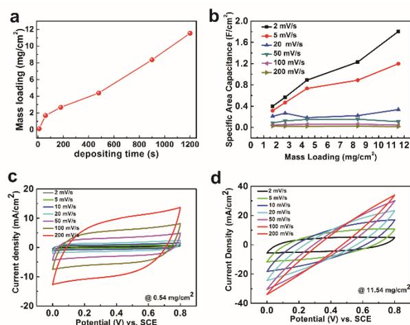
Fig. 3. (a) mass loading density of MnO<sub>2</sub> under gradually increasing electrodepositing duration. (b) Areal capacitance vs. mass loading for MNPC hybrid films at different scan rate. (c) Representative CV curves of MNPC hybrid film with mass loading of 1.7 mg/cm<sup>2</sup> (c) and 11.54 mg/cm<sup>2</sup> (d) at different scan rate.
