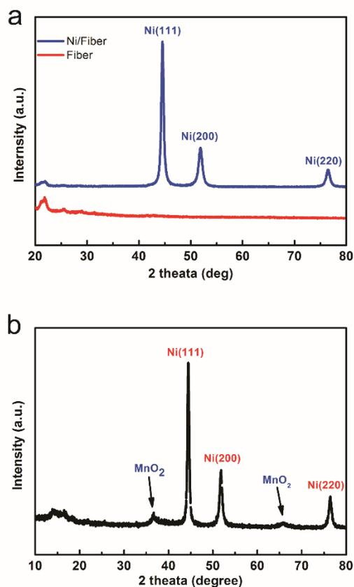
Fig. 1. (a) XRD pattern of polymer fiber and nickel coated polymer fiber membrane. (b) XRD pattern of MnO<sub>2</sub> deposited on NCP.
